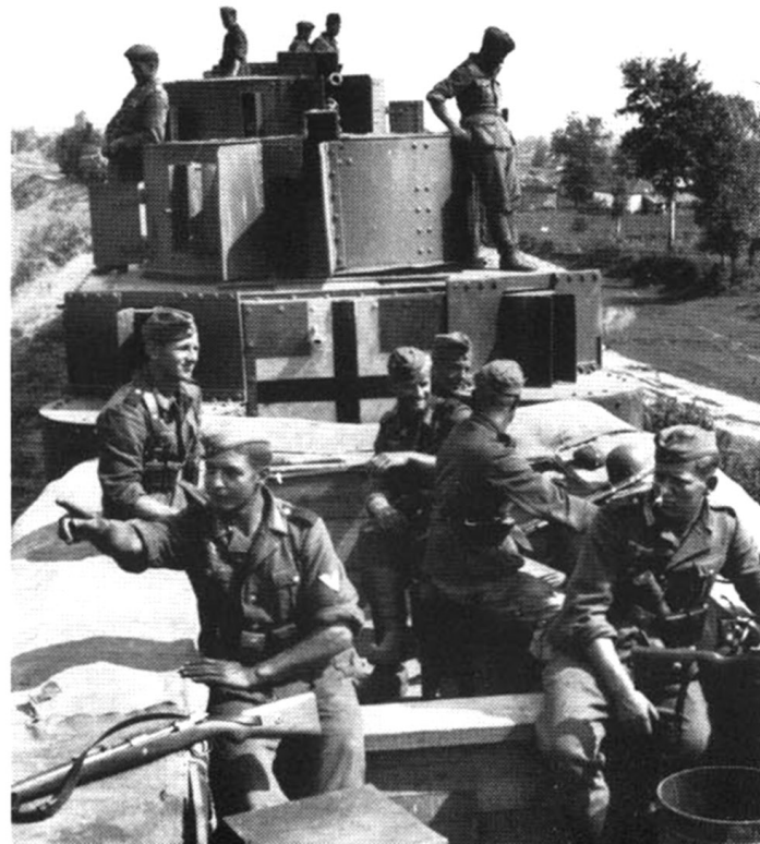
An auxiliary broad-gauge armored train (track-guarding train), manned by the 3rd Company of Railroad Engineer Regiment No. 3 in Kleist's armored unit (Southern Army Group), consisting of a Russian Type O armored locomotive (upper right), a captured two-turret artillery car, from which one cannon has been removed (lower left), and three low-board cars (with doubled walls of cast concrete or piled sandbags), manned by infantrymen, with a 3.7-cm antitank gun in front (lower right). (3 BA, 1 La).
