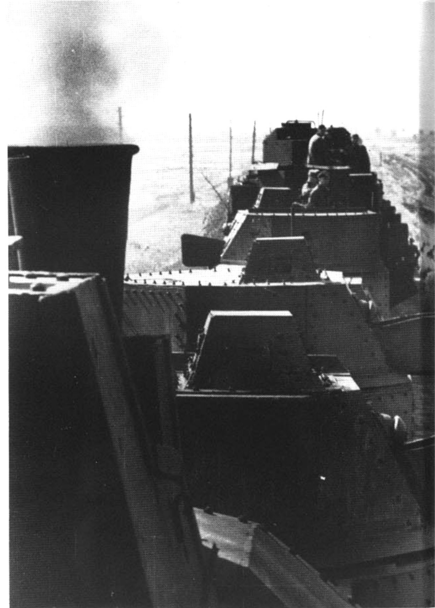
Another broad-gauge armored train made of captured Russian rolling stock. Its being armed with four guns (though by the thickness of their barrels they are smaller than the usual 7.62-cm caliber) shows it to be a regular armored train, perhaps of the reequipped 26-31 series, but a more precise identification based on this pictorial material is impossible for the time being. (3 x BA)
